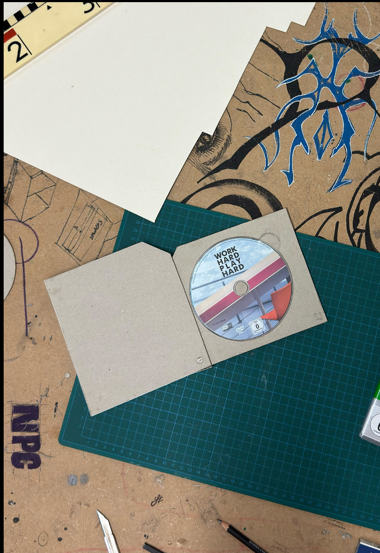
The innovative construction of the packaging relies entirely on a small rolled piece of paper in the bottom corner which ensures the inner board to move freely.
